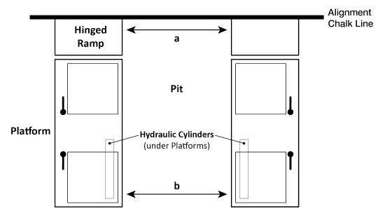
Make the Alignment Chalk Line longer than the width of the P-9000LT and the Pit.
