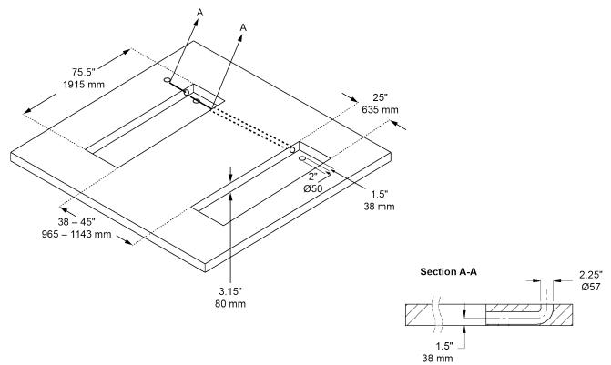
Depth of Concrete Cutouts must be 3.15 inches. There must also be 4.25 inches of concrete below the bottom of the Concrete Cutouts.
