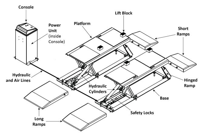
Covers for Hydraulic and Air Lines included with Lift. Optional Lift Arms not shown. P-9000LT **F** does not have Long or Short Ramps.
